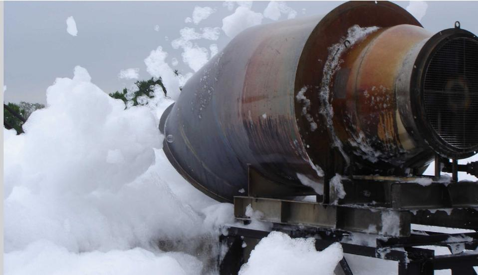
High expansion foam systems represent the most effective protection for LNG (Liquefied Natural Gas) spills, both for vapour reduction and dispersion as well as for radiant heat reduction and fire control.
